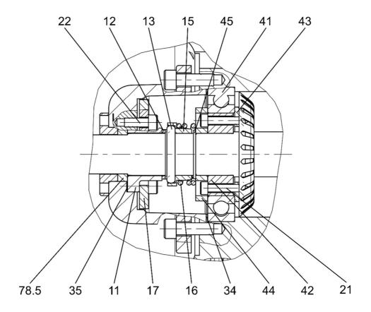
Figure 3d: Details of shaft seal
