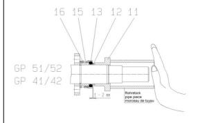
8. The O-ring must press the slide ring tightly onto the shaft. Therefore, use the loose slide flange (11) as an auxiliary tool.
