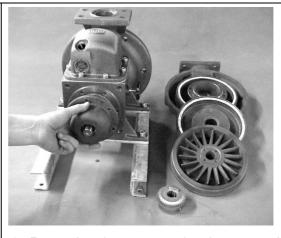
6. Removing the outer seal at the motor side
