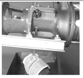
4. Drain oil in a suitable container.
