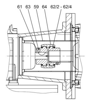
Figure 3c: Detail of coupling and motor connection
