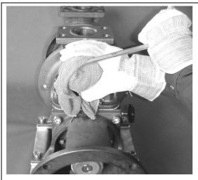
1. Carefully open the oil filler plug (57) ½ turn and wait until the oil chamber is depressurized (this may take a while!) Use a wet cloth to protect the plug.
