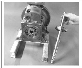
3. Push out shaft and inner bearing with a plastic hammer trough the housing.
