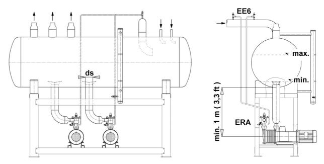
Fig.6 Application with two pumps in operation
