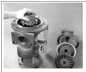
5. Dismanteling pump parts and inner seal at the pump side.
