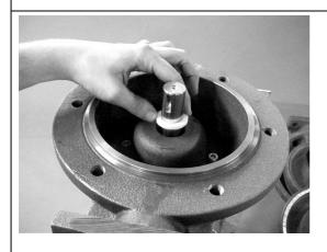
11. Fit for GP 50 pumps 1 felt ring respective for GP 40 pumps 2 felt rings (78.5) and assemble part 78.
