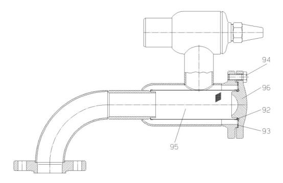
Figure 3e: Details of strainer KS 40-P / KS 50-P
