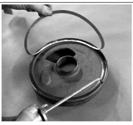
12. Lightly oil the grooves of the intermediate rings.
