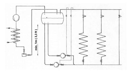
Fig. 4 principle of pump recirculation system
