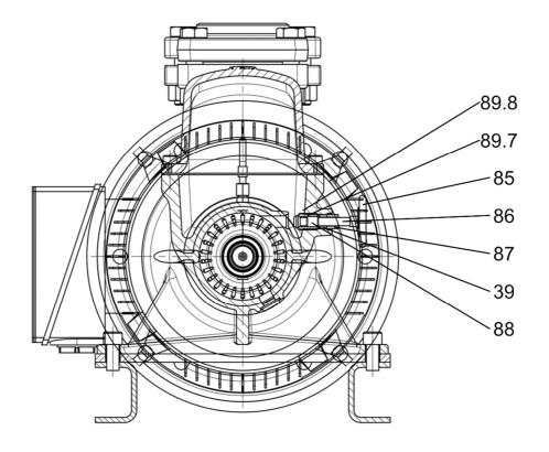
Figure 3b: Details of bearing
