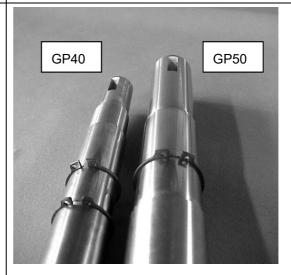
The bearing in GP 50 pumps is supported with only 1 snap ring. GP 40 pumps require 2 snap rings to fit the bearing.
