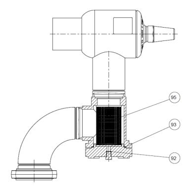
Figure 3f: Details of strainer KS 80-P
