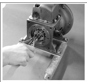
You can only remove the snap (Seeger) ring, if the screws in the tightening ring are loose!
