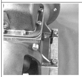
3. The hand wheel (85) must be completely open to ensure that the pressure may equalize between oil and pump chamber.
