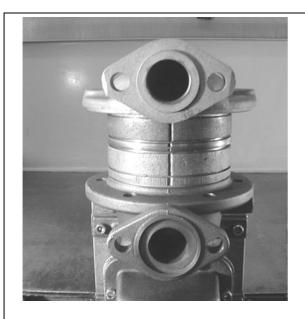
15. Assemble the intermediate rings and gaskets (33) in such a way that the marks align.
